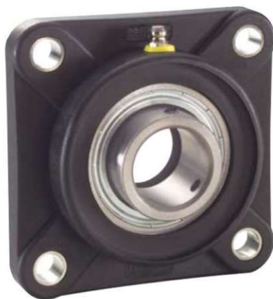
Flange bearing with solid housings series UCFC for plain shafts d 12-15-16-17-20-25-30-35-40 mm
