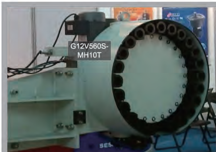
G12V560S-MH10T用於刀庫圖示 G12V560S-MH10T on ATC.
