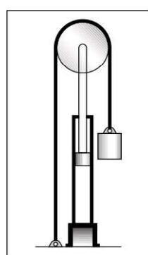
**Fig 3** - Suspension of the load on an overhead chain hoist. The chain meshes with a sprocket usually motor-power driven through gearing. The slack side of the chain generally hangs freely, thus providing 180° wrap on the sprocket. For application with frequent movement and shock loading at slow speeds. Hoist chains are frequently used in this application.
