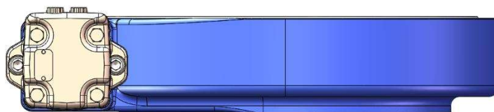
Horizontal installation, base downwards --- there is a risk of water ingress when used outdoors
