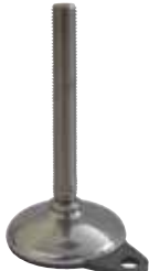
Part. R0747F - Pag. R037 Ø 80 • Stainless steel • Hygiene • Prefitting for fixing • Max. load 25000 N.
