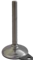
Part. R0748F - Pag. R37 Ø 100 • Stainless steel • Hygiene • Prefitting for fixing • Max. load 25000 N.
