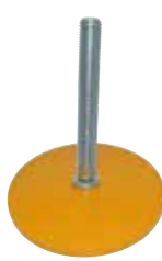
Part. R0408 - Pag. R35 Ø 160 • Painted steel • Max. load 50000 N.
